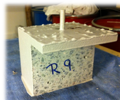
Epoxy coated concrete specimen
